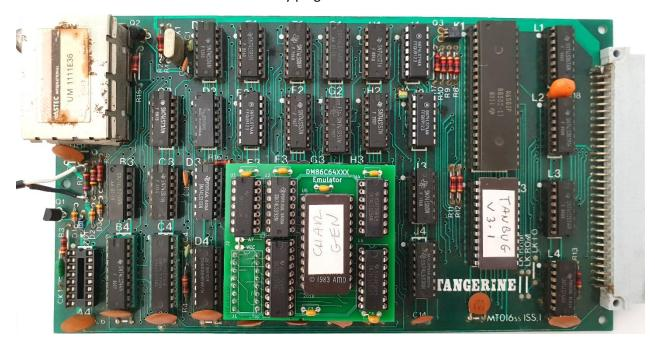
Check to ensure that nothing is protruding below the board that could cause a short circuit. It may well be prudent to apply some tape. For systems subject to movement double sided foam tape is recommended.
